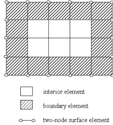
**Figure 1.** Schematic diagram of mesh map of solid containing surface elements.
