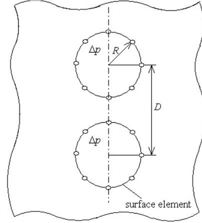
**Figure 3.** Schematic diagram of two nanovoids attached by surface elements in an infinite domain.
