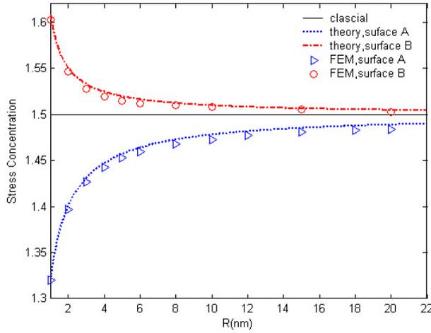
**Figure 2.** Variation of stress concentration with the void radius  $R$ .
