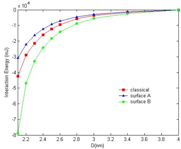
**Figure 5.** Variation of the interaction energy as the distance between two voids.
