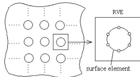
**Figure 6.** Schematic diagram of periodic arrays of nanoporous solid and RVE.
